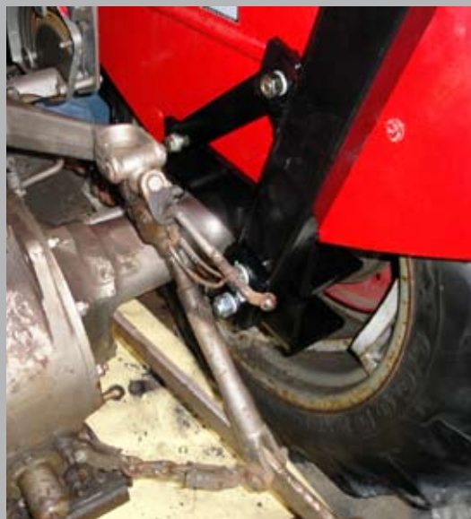
Steps 11-13 Installation of Right Vertical Tube Part 6R
