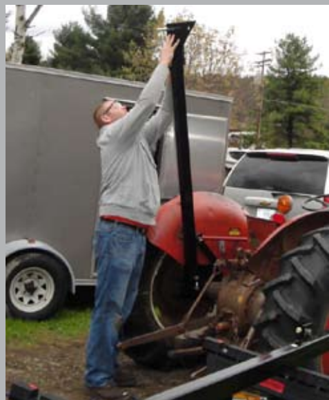
Steps 5-7 Installation of Left Vertical Tube Part 6L
